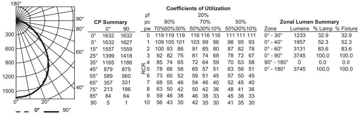
2GTL 4 40L LP835, 4006.7 delivered lumens, test no. LTL22798PO, tested in accordance to IESNA LM-79.
